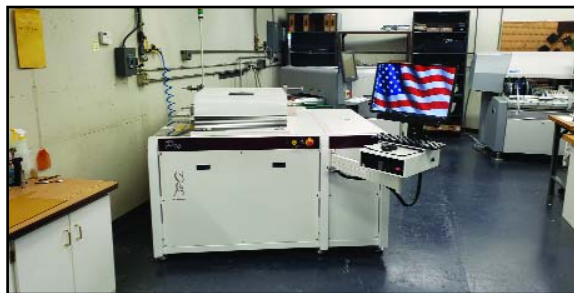
Pillarhouse Jade Pro offline selective solder system.
